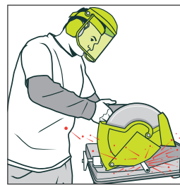
Figure 25: The self-adjusting guard over the cutting wheel swings back as the cutting wheel cuts through steel
